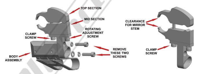
3 - The BODY ASSEMBLY must be removed to gain access to the CLAMP SCREW. Remove the two socket head screws as shown above. Be sure to remove the lock washer with the top screw along with the lock washer and flat washer with the bottom screw. Loosen the CLAMP SCREW so there is enough clearance between the TOP and MID SEC-TIONS to slide over the mirror stem. YOU MAY ADJUST THE MIRROR PARALELL TO THE WINDSHIELD AND SLIGHTLY UPWARD FOR EASE OF INSTALLATION.
