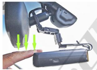
**7 -** If the RD is too close to the bottom of the mirror, You may access the buttons on top of the RD by gently pushing downward on the front of the RD with one finger and push the desired button with another finger. Then allow the RD to return to it's original position by gently letting it spring upward. When accessing the buttons, be sure to push the RD downward just enough for your finger to fit between the RD and mirror. **Do not push down more than what is needed.**
